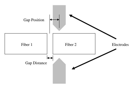
Arc power and duration allow the technician to apply varying amounts of power to the splice point. This may be necessary if the fibers are harder to melt and require more heat to melt the fibers. The arc power and duration can also be reduced to better control fiber melting.
