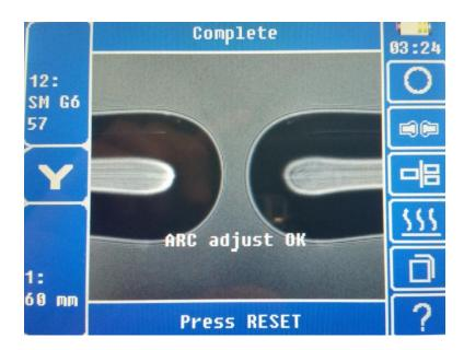
The shape of the fiber ends is analyzed to determine if the optimum power is applied. The process is iterative and requires that the technician repeats the step until the splicer reports back that the ARC power was successfully adjusted.
